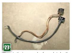
Wire protection is a personal preference, but a length of heatshrink over the twin 4mm-squared cables looks tidy. The ring terminal is also soldered in place. This is capable of a 78-amp nominal load. An electric heat gun is your friend for the heatshrink tubing.
