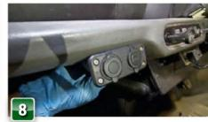
This surface-mount socket will either require a custom bracket to install it under the shelf...
