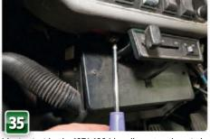
Moving inside, the 1976-1996 headlamp toggle switch is worthy of note. The full power of the headlamps surges through this plastic-bodied switch, so failure is not uncommon. To access it from behind, drop the heater down by undoing the two self tapping screws under the dash rail.
