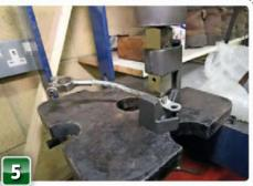
Large ring terminals such as this one need equally large crimping tools for a satisfactory crimp. 12 Volt Planet sells this budget tool, which works pretty well for occasional jobs, especially when used in a vice or press rather than simply smacking it with a large hammer.
