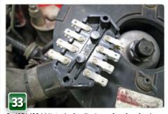
On 1976-1996 Minis, the familiar Lucas four-fuse fusebox is another common failure point to check ahead of the winter. The terminals frequently corrode from behind, causing all manor of unusual problems and annoyances. Removed from the bulkhead, test for high levels of resistance across the box with a multimeter.
