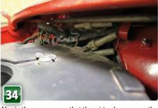
Also in the area, ensure that the wiring loom up on the bulkhead is not caught up on the air filter housing, pulled overly taught or in contact with any sharp edges or the bonnet hinges. On later cars with thick sound insulating material, the area can be quite congested with cabling and relays.
