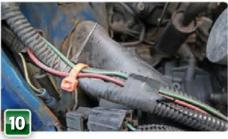
The convoluted plastic sleeve is there to protect the wiring insulation from cuts and the elements, so why someone has routed these wires outside of it is quite puzzling. It's messy, lazy and potentially dangerous if the wires have not been adequately fused. There's no added cost in spending a little more time to route everything safely.
