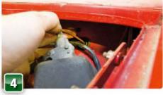
Feed the cable through the bulkhead in a suitable, neat location, remembering to protect it with a rubber wiring grommet.
