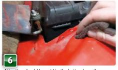
Attention should be paid to the battery's earth connection on the boot floor, keeping it free of paint and rust. With excessive strains placed upon the battery from an insufficient charging system, or if the battery is not earthing to the body effectively, accelerated corrosion of the earth strap can occur from the excess heat of electrical resistance.
