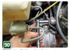
It's more beneficial to replace the top engine steady earth strap if that's in poor condition. The bolt here was quite loose, giving a poor electrical contact, and not to mention the high likelihood of shearing it off in the block.
