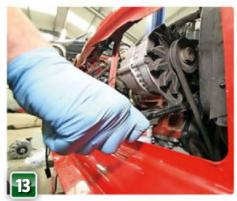
With the battery disconnected, the grille removed and the alternator plug released, begin by loosening the lower adjustable bracket fixings.
