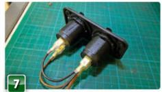
Because we're dealing with a dual socket, it requires two live and two earth terminals. You can piggy-back the connections from one to the other, again ensuring sufficient cable gauge for the job.
