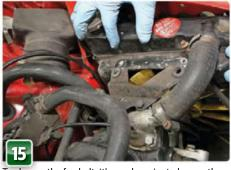
To change the fan belt, it's much easier to loosen the top radiator bracket fixings and one of the top hose clips and give yourself a little extra clearance. Be careful not to fully remove the top hose from the thermostat housing, or you may loose coolant.
