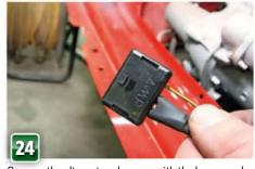
On goes the alternator plug cap, with the brown and yellow charge light wire similarly soldered to a new terminal. When you're building a wiring loom from scratch, it's nice to heatshrink all three cables together, but here the charge light disappears off into the loom, making that rather awkward in situ.
