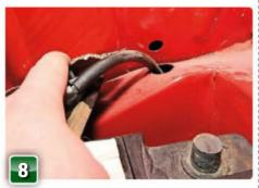
This car was missing the essential rubber grommet on the live cable. The insulation around the main power cable might be thick, but a sharp edge like this will soon cut into it, shorting on the battery and in all likelihood, setting your pride and joy alight.
