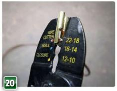
A new alternator plug was also sourced, which comes with fresh non-insulated 90-degree spade terminals. These are a tad awkward to crimp with ratchet-type tools, but the basic ones are adequate.
