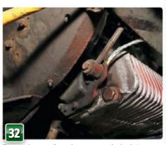
Two earth straps from the engine to the body/ subframe are recommended. The lower front engine steady is a convenient point on this car.
