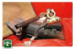
Equally nasty are these screw-in battery clamps. The cable crushes down unevenly and can loosen over time. Here the clamp's fixing bolt has even been omitted, perhaps due again to unsuitable battery selection. Battery terminal poles are not standardised in dimension, so check carefully before you buy.
