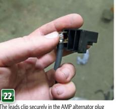
The leads clip securely in the AMP alternator plug from behind.
