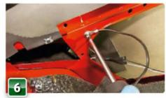
Now we need to fit an earth. Screwing a ring terminal to a suitable point under the dash rail will suffice. Test the earth cable's connection with a 12-volt multimeter or circuit tester.
