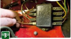
On a standard car, feeding from a spare fused ignition-live terminal on the fuse box makes sense. Check your workshop manual's wiring diagram to see which feed may be best suited. If in doubt, always install an extra in-line fuse.
