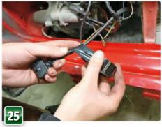
That said, you can still wrap the new loom section up in tape. Use adhesive PVC tape to stick down the ends of non-adhesive tape and follow it up the loom for protection.
