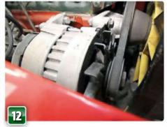
With increased use of the lights and heater comes extra strain on the alternator. This unit had developed a fault and was no longer charging sufficiently. The drive belt is also clearly in need of replacement.
