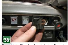
The switch itself is quite robust, but the addition of extra lights to the standard circuit, or a bodged installation somewhere along the line, means that they can quickly overheat and short out. If in doubt, install a four-way 12-volt relay for your additional lighting, or run a separate ignition-live switched feed.
