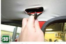
Another potentially dangerous issue spotted on this car was the interior light. I'd planned to recommend lower ampage LED units to reduce demand on the electrics, but here it was missing entirely. The connector is a permanent live feed, and although fused, needs better insulation if disconnected.
