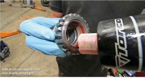
including AC Dodd, seemed positive that that could finally be the answer. And that was it, after days of struggling. Our mechanic Matt gave me a hand to clean up the bush and crankshaft tail on which it spins, we applied some cam lube and the clutch was finally disengaging again. So two problems that were really confusing matters, but at least I've learnt everything there is to know about pre-Verto clutches!
