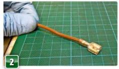
We'd recommend non-insulated crimp terminals with the separate rubber sleeves for the most secure connection. Additional solder here would probably give the ultimate terminal.
