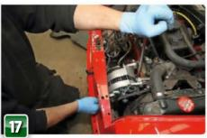
Check that the new belt is the correct length for the job. The water pump pulley varies in diameter, so not all fan belts are equal, hence why we have temporarily refitted the old one, as the replacement was too short. Apply tension to the belt with a large spanner as you tighten the fixings all round.
