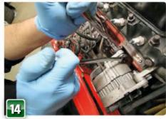
Access is much easier up top for the 1/2-inch AF bolts. Once these and the 9/16inch AF fixing on the sliding bracket below all are loosened it will be straightforward to remove the fan belt from the pulle and carefully extract the alternator.
