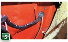
We found a handy location already on the bulkhead to pass the cable through. Move the interior sound deadening to carefully pull the cable from inside.
