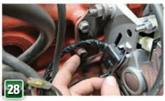
Most alternators do not come with a new spring clip for some reason, so you'll need to reuse the old one to hold the plug securely in place. That's not the only aspect to the charging system, however. Earths and the live feed itself should also be considered. Sound-off competitors regularly upgrade the main battery feed for a larger gauge cable.
