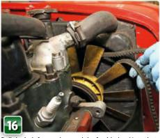
Pull the belt free and around the fan blades. Note that someone has also installed the fan blade back to front here - the next job on the 'to do' list...
