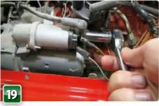
Double check the battery earth is disconnected and remove the nut securing the brown alternator feed to the starter solenoid, here on the starter itself. Earlier inertia-type starters have their solenoid on the offside inner wing. The process is the same, although slightly less fiddly with a later pre-engaged set-up.
